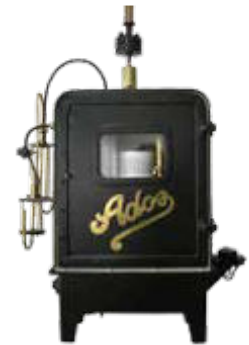
A test instrument hanging in a universal joint (to compensate the strong wave motion on board of a ship), when measuring carbon dioxide.
