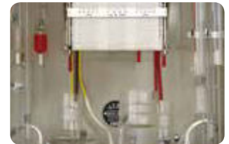
Triple test instrument (Triplex) for monitoring the CO, H 2 and CO 2 content of the ambient air. Used in the chemical industry.
